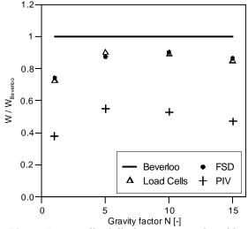
**Figure 7.** Normalised discharge rates, Polyamide in silo with flat bottom
