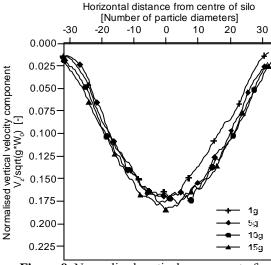
Figure 9. Normalised vertical component of velocity during discharge with glass beads in silo with flat bottom
