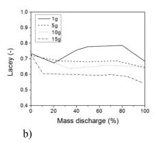
**Figure 20:** Lacey index of the evolution of the segregation state in the silo – (a) Glass beads flat bottom - (b) Glass beads 30 degree hopper
