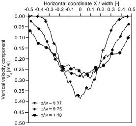
**Figure 16.** Flow profiles at different heights for Glass beads in silo with flat bottom at 10g
