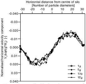
**Figure 13.** Normalised horizontal component of discharge velocity for glass beads in silo with flat
