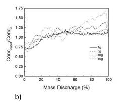
**Fig 19:** Segregation propensity of the mixture (Conc. outlet of the coarser particles index vs. mass discharge) for 1g, 5g 10g and 15g. (a) Glass beads – Flat bottom (b) Glass beads – 30 degree hopper
